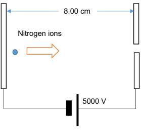
a) Calculate the electric field strength between the parallel plates.
